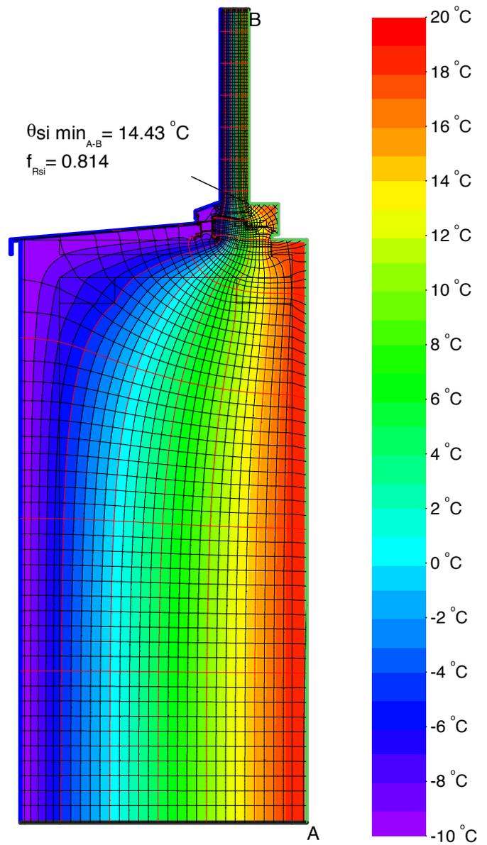
$$\Psi_{A-E,C} = \frac{\Phi}{\Delta T} - U_1 \cdot b_1 - \frac{\Phi_2}{\Delta T} = \frac{13.313}{30.000} - 0.131 \cdot 1.010 - \frac{8.312}{30.000} = 0.034 \text{ W/(m} \cdot \text{K)}$$
