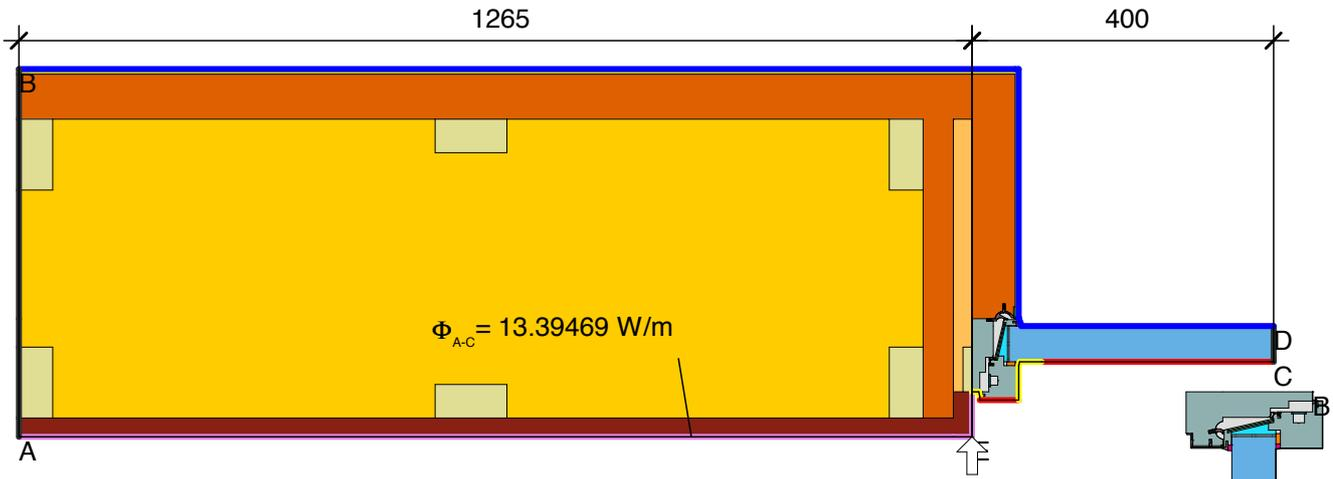
$$\psi_{A-E-C,*} = \frac{\Phi}{\Delta T} - U_1 \cdot b_1 - \frac{\Phi_2}{\Delta T} = \frac{13.395}{30.000} - 0.132 \cdot 1.265 - \frac{8.124}{30.000} = 0.009 \text{ W}/(\text{m} \cdot \text{K})$$
