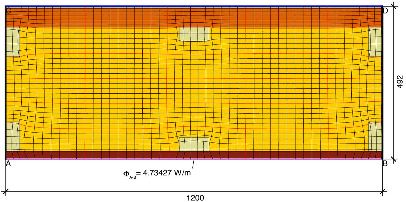
$$U_{\text{eq A-B}} = \frac{\Phi}{\Delta T \cdot b} = \frac{4.734}{30.000 \cdot 1.200} = 0.132 \text{ W}/(\text{m}^2 \cdot \text{K})$$
