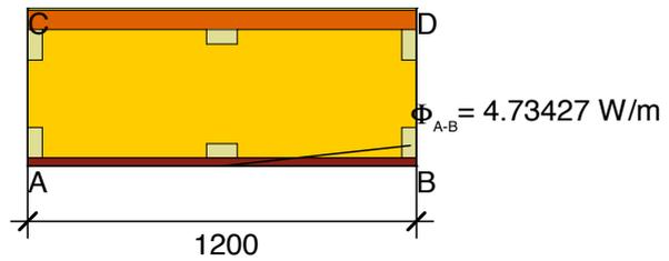
$$U_{eq\ A-B} = \frac{\Phi}{\Delta T \cdot b} = \frac{4.734}{30.000 \cdot 1.200} = 0.132 \text{ W}/(\text{m}^2 \cdot \text{K})$$
