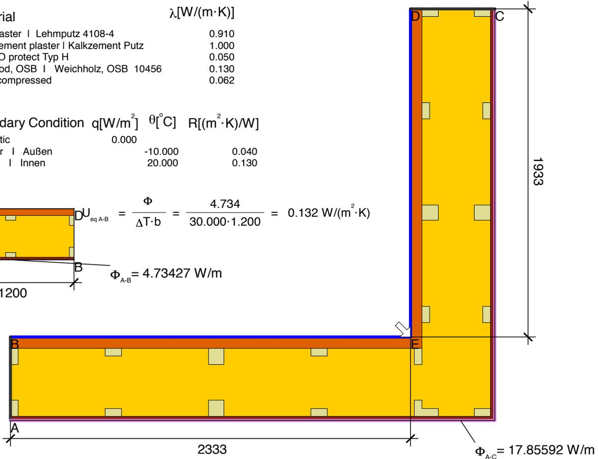
$$\psi_{A-E-C} = \frac{\Phi}{\Delta T} - U_1 \cdot b_1 - U_2 \cdot b_2 = \frac{17.856}{30.000} - 0.132 \cdot 2.333 - 0.132 \cdot 1.933 = 0.034 \text{ W/(m} \cdot \text{K)}$$
