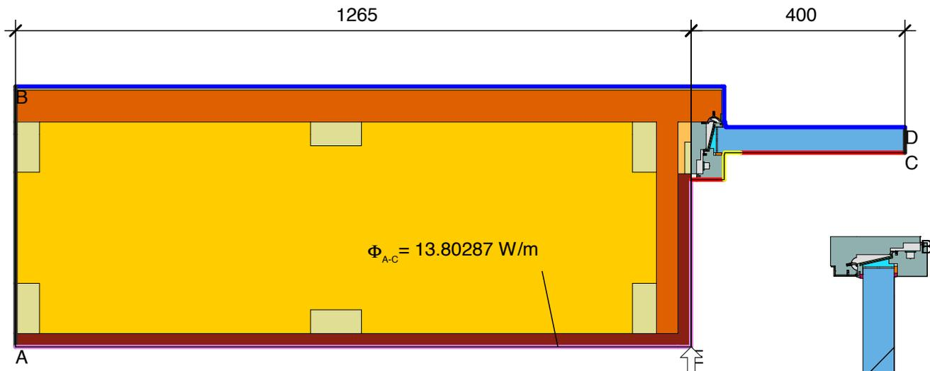
$$\psi_{A-E,C,*} = \frac{\Phi}{\Delta T} - U_1 \cdot b_1 - \frac{\Phi_2}{\Delta T} = \frac{13.803}{30.000} - 0.132 \cdot 1.265 - \frac{8.124}{30.000} = 0.023 \text{ W}/(\text{m} \cdot \text{K})$$
