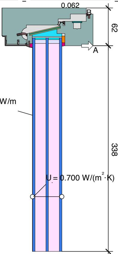
$$\psi_A = \frac{\Phi}{\Delta T} - U_g \cdot b_g - U_f \cdot b_f = \frac{9.237}{30.000} - 0.700 \cdot 0.338 - 0.831 \cdot 0.062 = 0.020 \text{ W/(m}^2 \cdot \text{K)}$$
