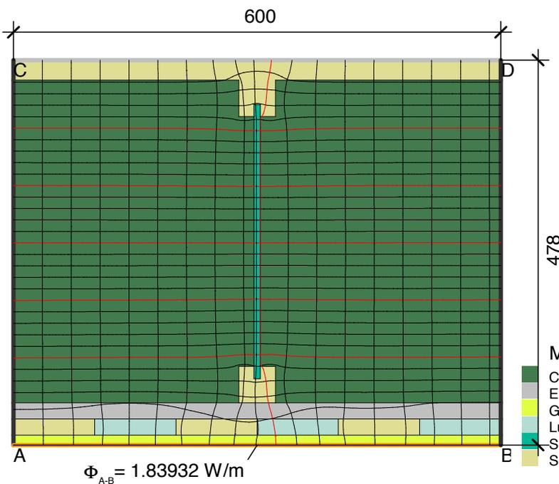
$$U_{\text{eq A-B}} = \frac{\Phi}{\Delta T \cdot b} = \frac{1.839}{30.000 \cdot 0.600} = 0.102 \text{ W}/(\text{m}^2 \cdot \text{K})$$
