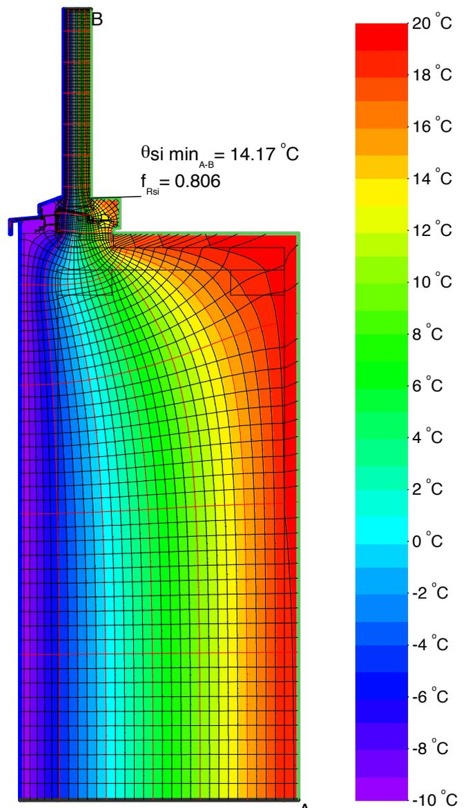
$$\psi_{A-E,C} = \frac{\Phi}{\Delta T} - U_1 \cdot b_1 - \frac{\Phi_2}{\Delta T} = \frac{13.307}{30.000} - 0.131 \cdot 1.010 - \frac{8.312}{30.000} = 0.034 \text{ W/(m}\cdot\text{K)}$$
