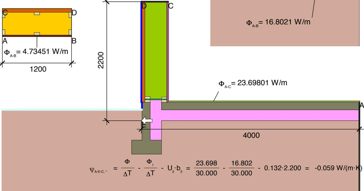
$$\psi_{\text{A-E-C}} = \frac{\Phi}{\Delta T} - \frac{\Phi_1}{\Delta T} - U_2 \cdot b_2 = \frac{23.698}{30.000} - \frac{16.802}{30.000} - 0.132 \cdot 2.200 = -0.059 \text{ W}/(\text{m} \cdot \text{K})$$
