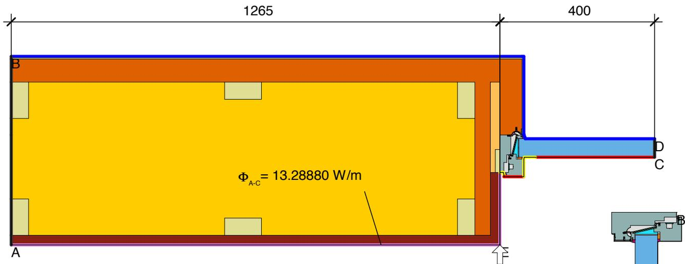
$$\psi_{A-E-C,*} = \frac{\Phi}{\Delta T} - U_1 \cdot b_1 - \frac{\Phi_2}{\Delta T} = \frac{13.289}{30.000} - 0.132 \cdot 1.265 - \frac{8.124}{30.000} = 0.006 \text{ W}/(\text{m} \cdot \text{K})$$
