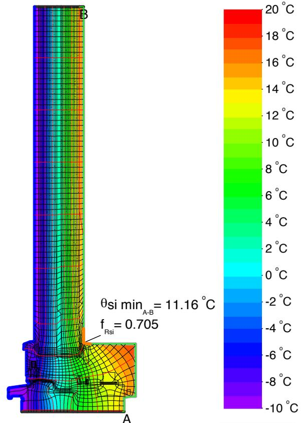
$$\psi_A = \frac{\Phi}{\Delta T} - U_g \cdot b_g - U_f \cdot b_f = \frac{9.671}{30.000} - 0.700 \cdot 0.333 - 1.028 \cdot 0.067 = 0.020 \text{ W/(m}^2 \cdot \text{K)}$$
