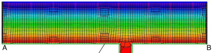
$\theta_{\text{si min}}_{A-B} = 18.83 \text{ }^\circ\text{C}$
