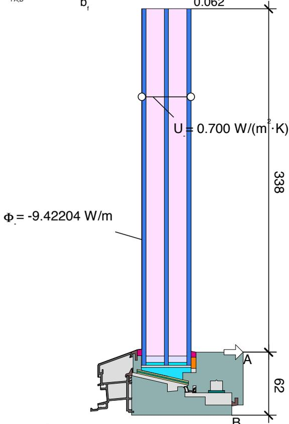
$$\psi_A = \frac{\Phi}{\Delta T} - U_g \cdot b_g - U_f \cdot b_f = \frac{9.422}{30.000} - 0.700 \cdot 0.338 - 0.932 \cdot 0.062 = 0.020 \text{ W}/(\text{m} \cdot \text{K})$$
