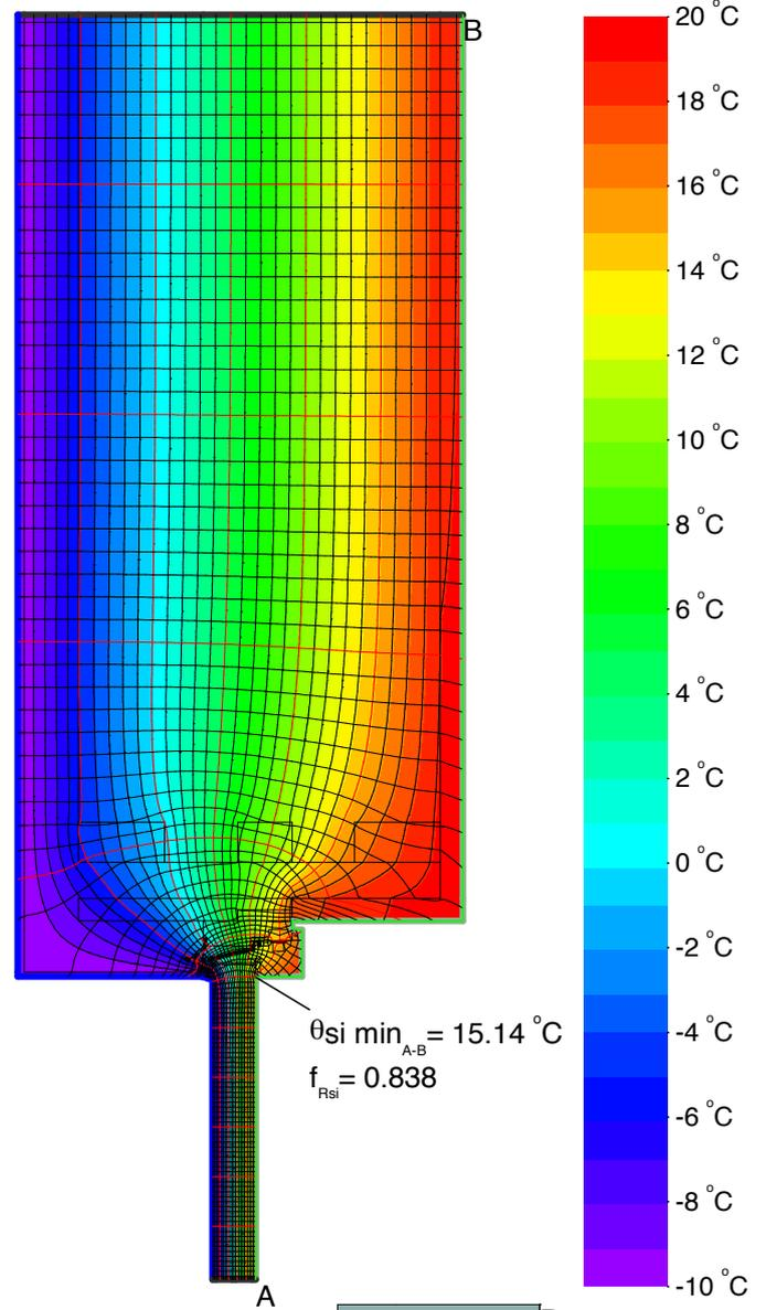
$$\psi_{A-E.C.} = \frac{\Phi}{\Delta T} - \frac{\Phi_1}{\Delta T} - U_2 \cdot b_2 = \frac{12.369}{30.000} - \frac{8.124}{30.000} - 0.131 \cdot 1.010 = 0.009 \text{ W}/(\text{m} \cdot \text{K})$$
