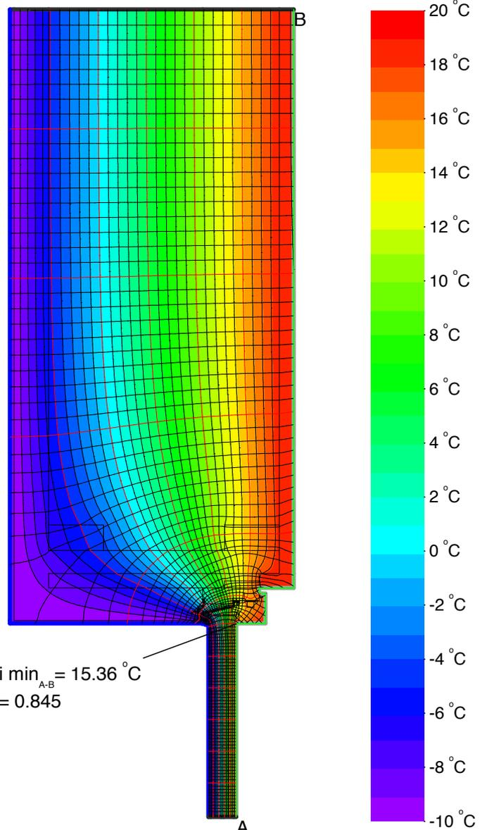
$$\Psi_{A-E-C} = \frac{\Phi}{\Delta T} - \frac{\Phi_1}{\Delta T} - U_2 \cdot b_2 = \frac{12.442}{30.000} - \frac{8.124}{30.000} - 0.131 \cdot 1.010 = 0.011 \text{ W}/(\text{m} \cdot \text{K})$$
