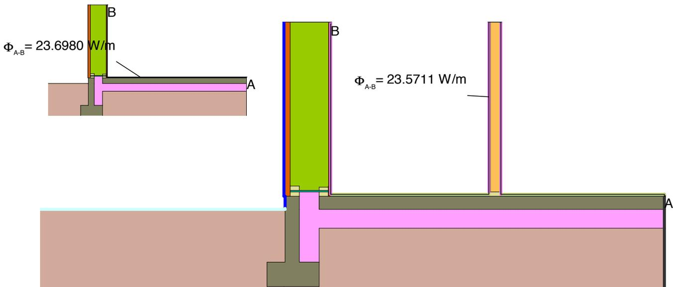
$$\Psi_{FSIW01} = (Q_{FSIW01} - Q_{FSEW01}) / \Delta\theta = (23,8711 \text{ W/m} - 23,698 \text{ W/m}) / 30 \text{ K} = -0,004 \text{ W/(mK)}$$
