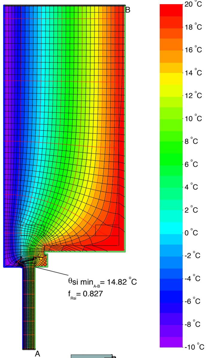
$$\psi_{A-E-C,*} = \frac{\Phi}{\Delta T} - \frac{\Phi_1}{\Delta T} - U_2 \cdot b_2 = \frac{12.844}{30.000} - \frac{8.124}{30.000} - 0.131 \cdot 1.010 = 0.025 \text{ W}/(\text{m} \cdot \text{K})$$
