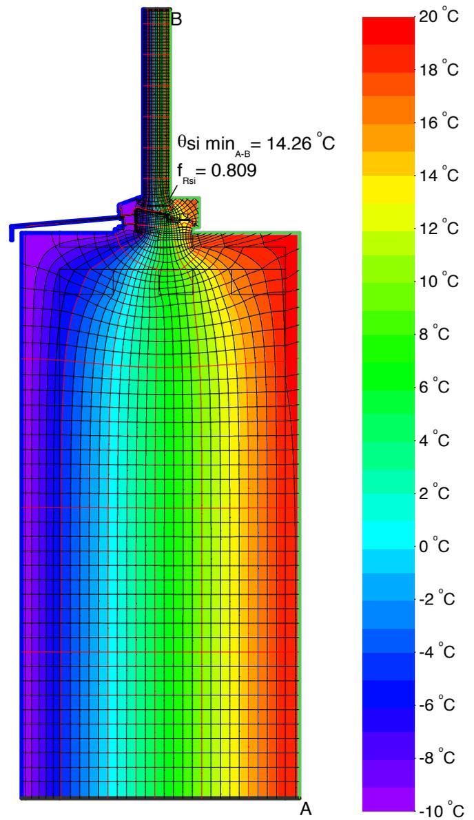
$$\psi_{A-E,C} = \frac{\Phi}{\Delta T} - U_1 \cdot b_1 - \frac{\Phi_2}{\Delta T} = \frac{13.087}{30.000} - 0.131 \cdot 1.010 - \frac{8.312}{30.000} = 0.026 \text{ W/(m}\cdot\text{K)}$$
