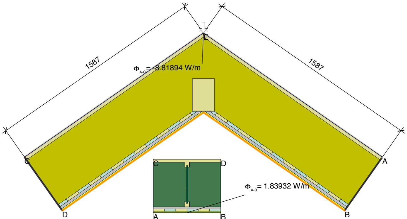
$$U_{\text{eq A-B}} = \frac{\Phi}{\Delta T \cdot b} = \frac{1.839}{30.000 \cdot 0.600} = 0.102 \text{ W}/(\text{m}^2 \cdot \text{K})$$
