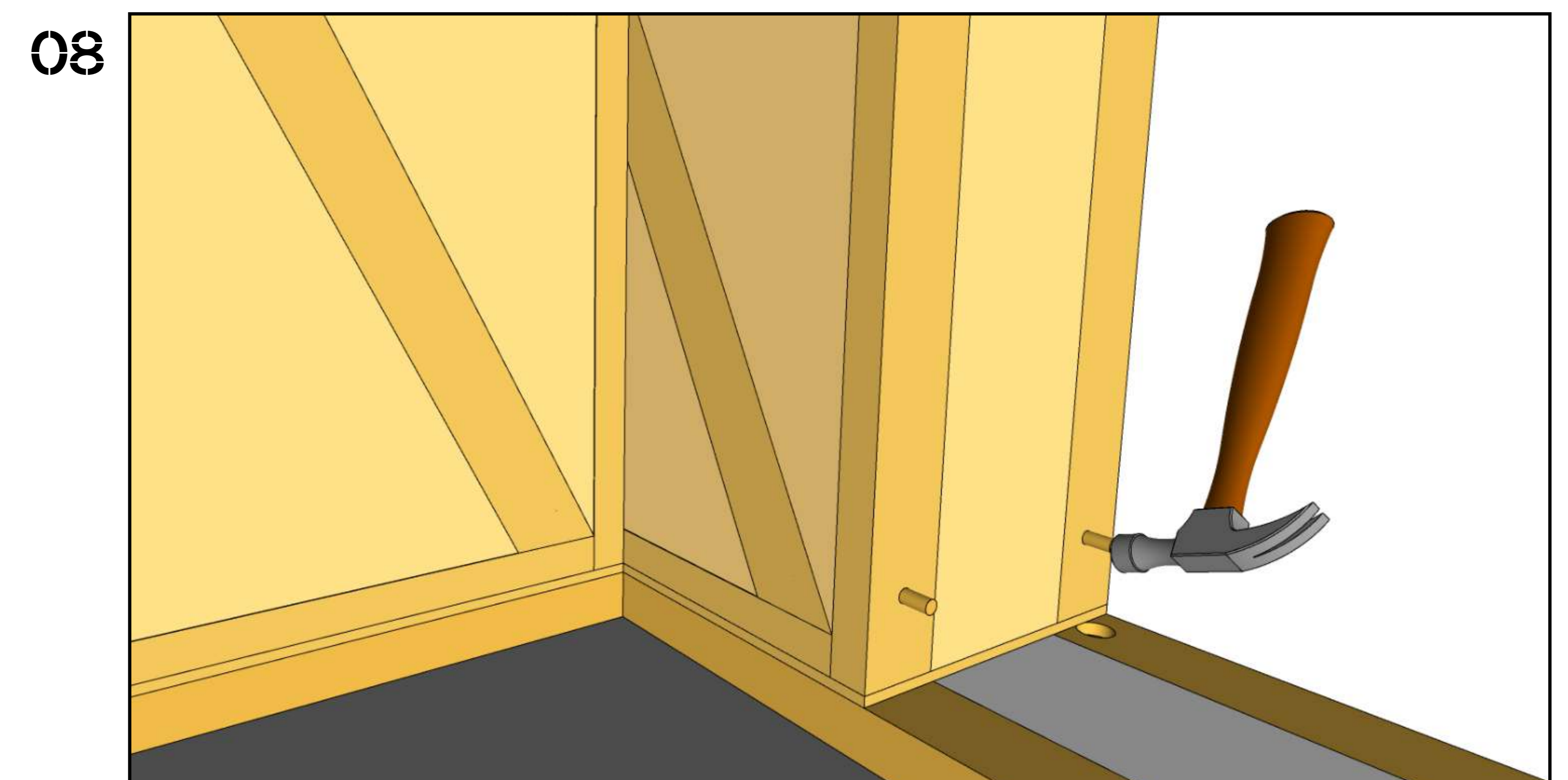
Insert the dowels into the holes to ensure exact connection.
