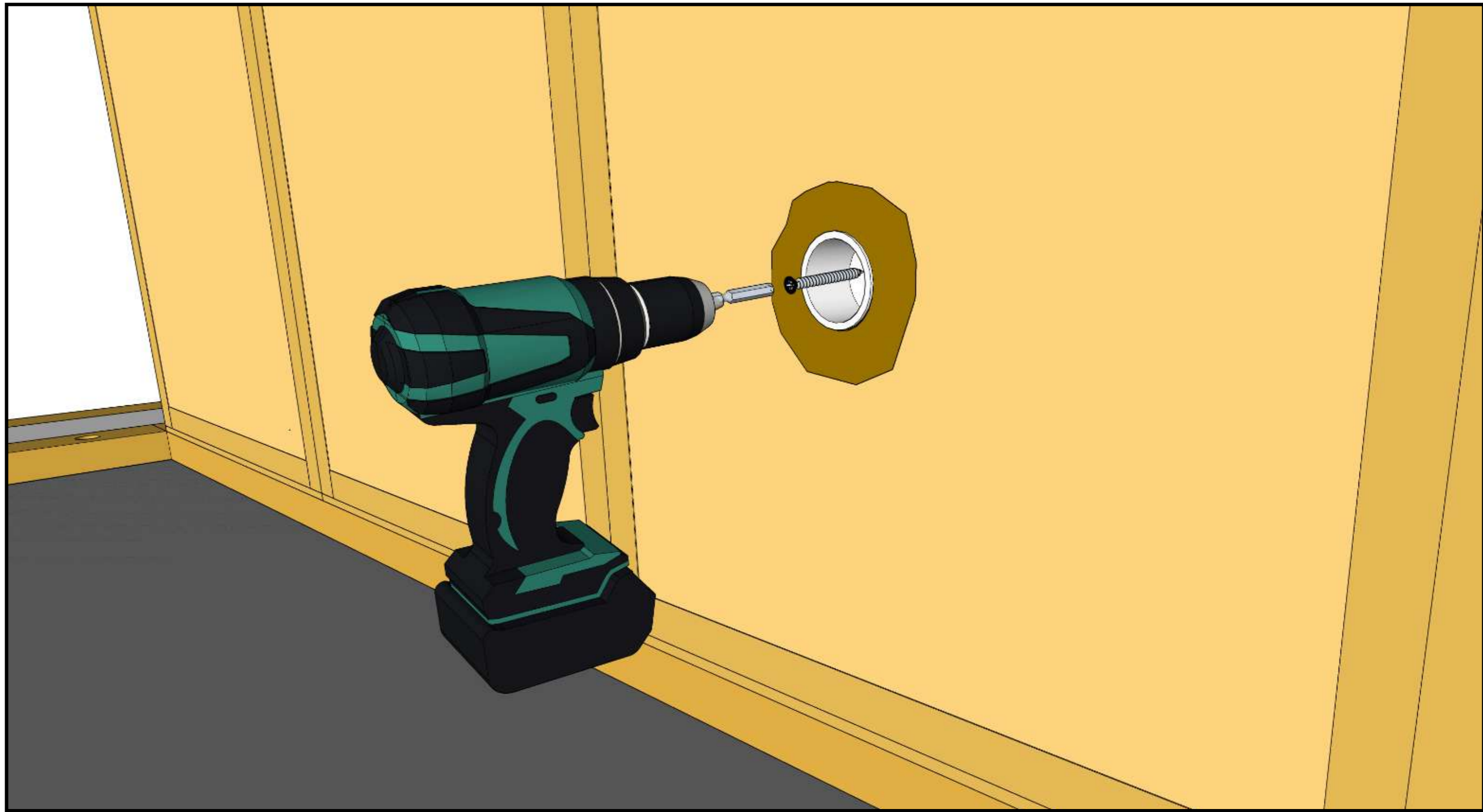
Fix the socket with a screw into the peg.
