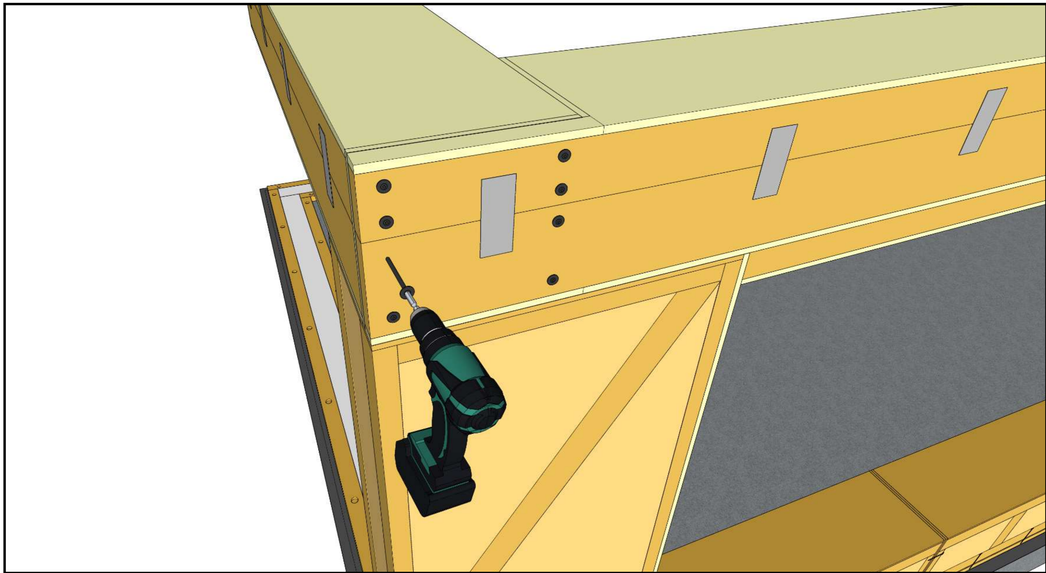
Screw the extended plywood piece of one Box element to the side of the other.
